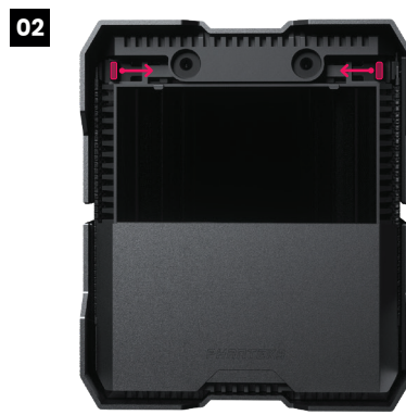
Slide the locks inwards to unlock.
