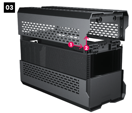
Slide the top panel to the front (1) and lift the top panel up with two hands (2).
